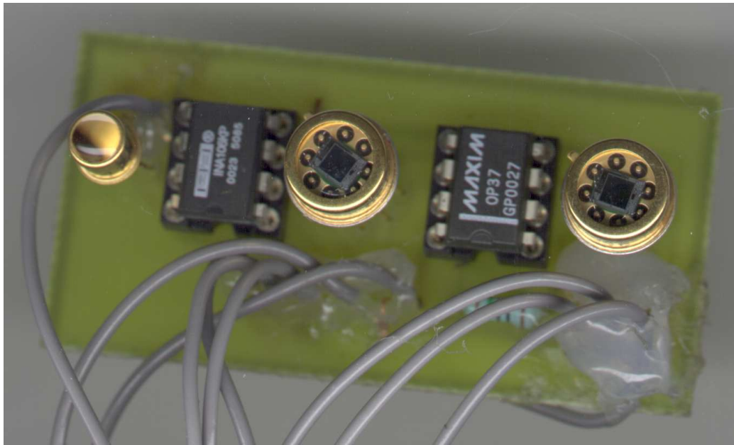
Figure 2.7: Finished PCB with components
